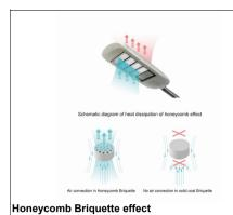
It simulates and adopts the burning principle of honeycomb briquette; it is easy to transform the original block of radiator to various modules, as well as to enable air to convect and fully pass through the gaps between modules by utilizing the honeycomb effect, thus to remove the heat rapidly, and reduce temperature by around 20 °C.
